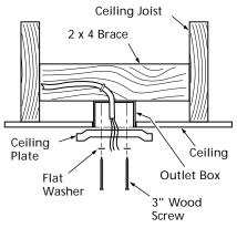
Figure 2c - Attaching Ceiling Plate to 2 x 4 Brace
